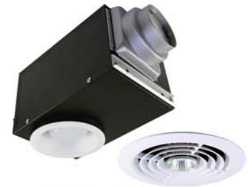
SE RVL-NM (No motor) 6" recessed down light with 15 watt GU-24 / R-30 fluorescent lamp and universal 4 & 5" duct adaptor. Includes bar hangers. Also available with 10 watt LED GU-10 lamp
